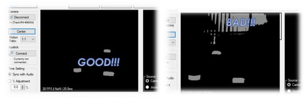
For best results, be sure to check that your head movements remain within the display window. If not, move back, away from the camera.
