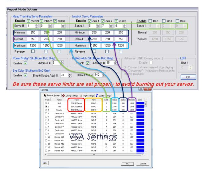
The [Power 'Relay' Setting] option is used when specific DMX controllers (such as the Skulltronix Board of Chuckee) have a specific address used to turn ON and OFF power to the servos. Consult your servo controller if this is required.
