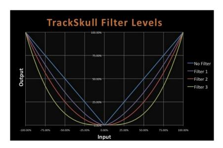
For example: Filter level 3 requires you to move almost 20% before any movement is seen by TrackSkull.
